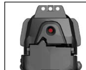
Figure 11 — Firing pin cocked
