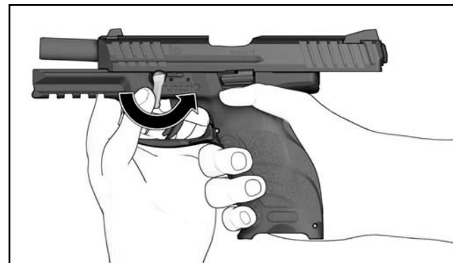
Figure 28 — Pivot the disassembly lever counter clockwise
