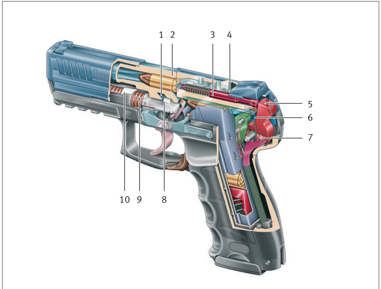
Fig. 13a: CDA trigger variant, cutaway view
