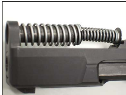
FIGURE 22.4: Spring correctly seated
